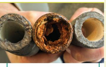
The water that leaves water treatment plants typically does not contain lead, but lead can be released into drinking water from corrosion in lead service lines and household plumbing that contains lead. If present, elevated levels of lead can cause serious health and development problems, especially for pregnant women and young children.
